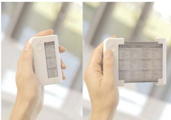
*Polymer Vision's READIUS™ can unroll its display to a scale larger than the device itself. (Courtesy of Polymer Vision / Philips).*
