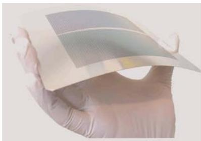
*Processing of low-temperature poly-silicon (LTPS) on metal foil
