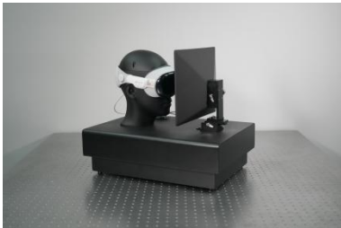
Figure 4. PTP Latency Measurement Device
