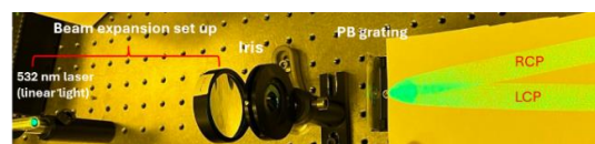
Figure 4. Experimental system for testing the PB grating.
