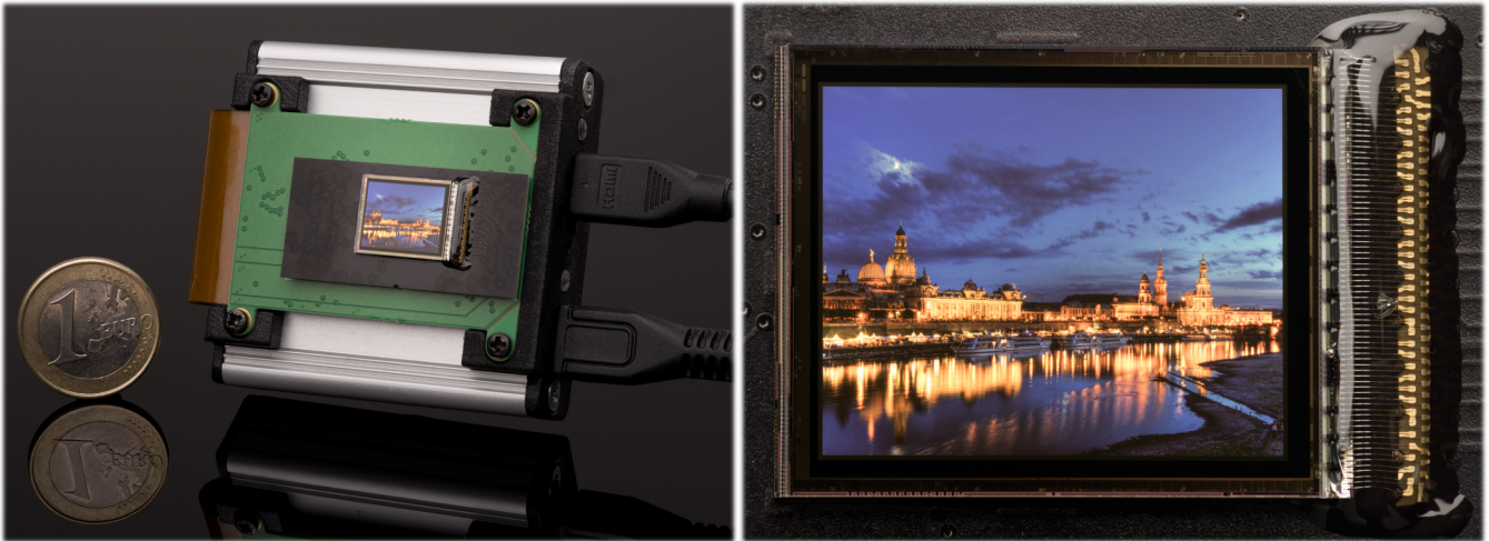
Figure 1. New high-voltage SXGA microdisplay on HDMI evaluation kit (left), closeup of microdisplay chip (right)
