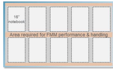
Figure 10. low glass utilization for FMM OLED
