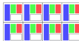
Figure 12. 4 th subpixel can be used for UPC or sensor integration
