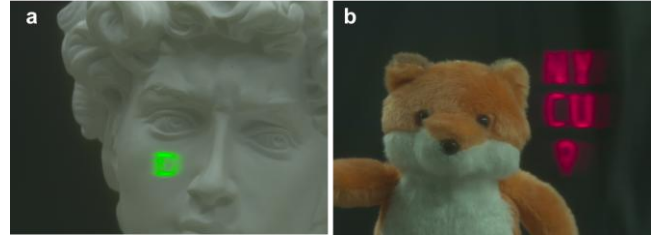
Figure 5. Demonstration of an AR platform utilizing a high- Q metasurface as the optical combiner. (a) An AR image showing the fusion of the real-world statue of David with a virtual label "D". (b) An AR image showing the fusion of the real-world fox plush toy with a virtual geolocation marker "NYCU."
