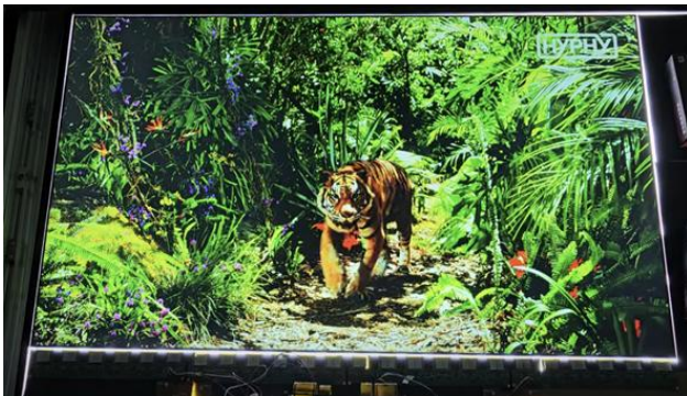
Figure 5: 65" 8K LCD panel driven by HYPHY HY1002 DDIC
