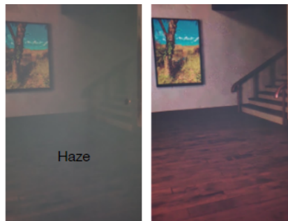
Figure 4. Quest 2 without CADC (left) vs. Quest 3S with CADC (right)
