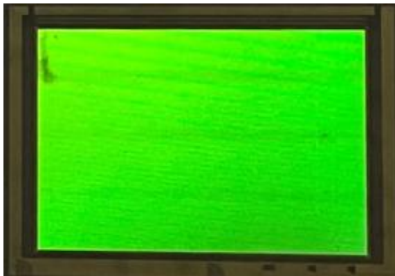
Figure 5. A picture of 2.5-inch 80 ppi AMOLED display.
