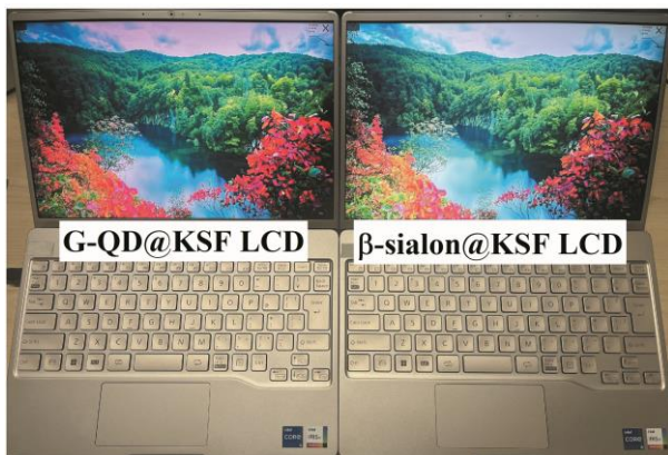
Figure 8. Comparison of digital images displayed by \beta -sialon@KSF LCD notebook and G-QD@KSF LCD notebook.
