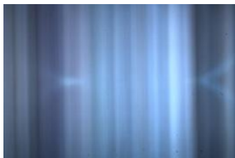
Figure 3. The luminance distribution of the eye box. The overlapping part, i.e. the eye box boundary, is difficult to distinguish.
