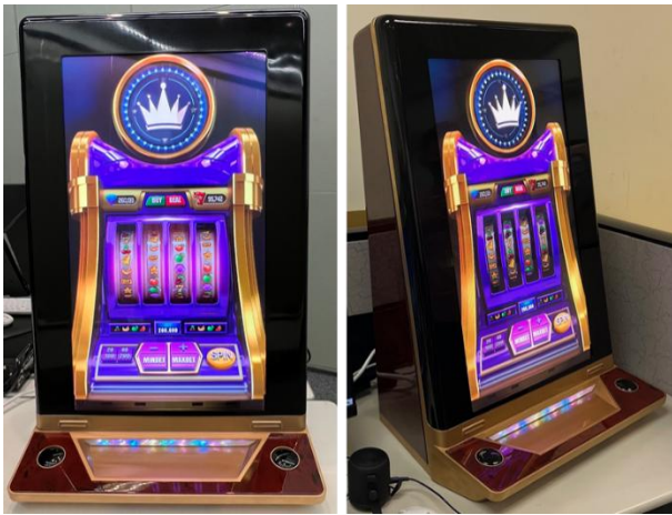
Figure 5. The 30" MLD panel uses transparent Micro LED and A.R.T. LCD to provide a true 3D experience for multiple viewers without wearables, even at varying distances and angles.
