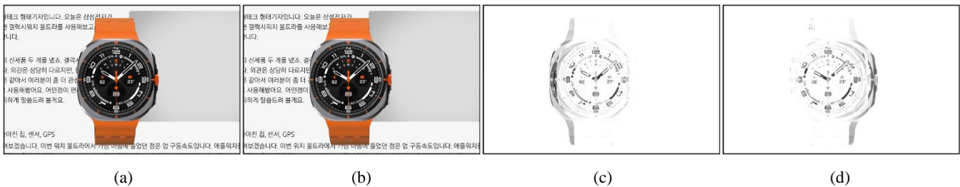
Figure 3. Examples of generating the color similarity maps: (a) Left perspective view image, (b) right perspective view image, (c) color similarity map of left image, and (d) color similarity map of right image. In color similarity maps, brighter areas indicate where the left and right images have similar colors; darker areas indicate where they have different color.
