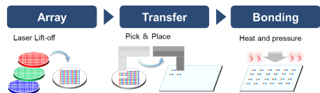
Figure 2. Micro-LED mounting process
