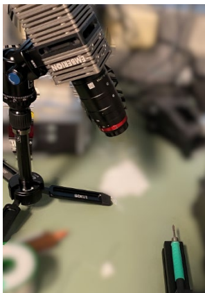
Figure 3 Experimental set up of the SWIR camera imaging a soldering iron
