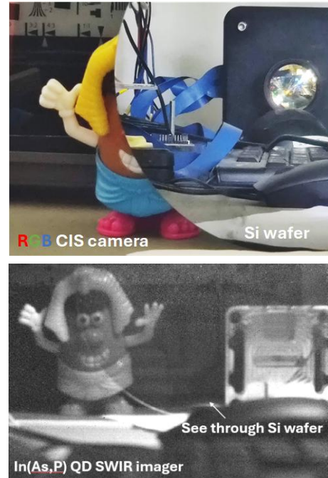
Figure 7. Proof-of-concept InAs image sensor for the SWIR range: test scene acquired with a CMOS camera (top); and InAs QD image (bottom).
