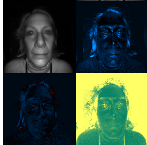
Figure 4: Image of subject under illumination, showing polarization birefringence and details. (Top-left): NIR intensity image (top-right): S1 polarization (bottom-left): S2 polarization, (bottom-right): Degree of linear polarization.
