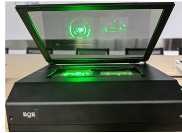
Figure 7. HUD optical system.
