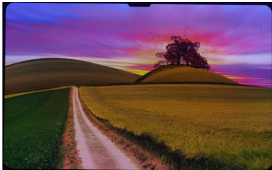
Figure 7. 13.2 inch full oxide AMOLED display with high mobility MO-1 metal oxide TFT backplane technology.
