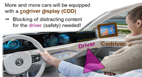
Figure 1. Visualization of automotive switchable privacy: The image on the codriver display is blocked to the driver if distracting content is shown. Source: Continental.
