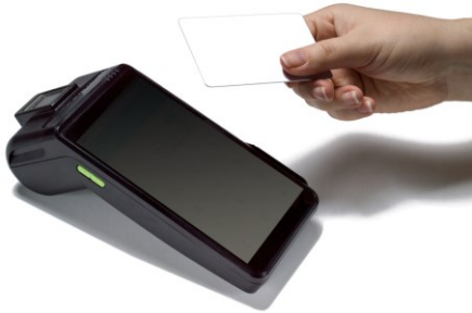
Figure 9. Shipping 5.8" POS privacy display incorporating BEF backlight stack and GH-SLCR
