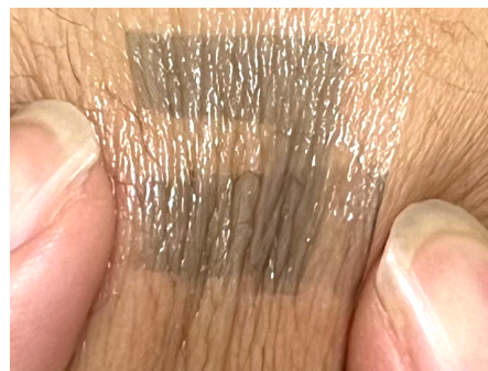
Figure 9. A highly skin-conformable piezoelectric sensor.
