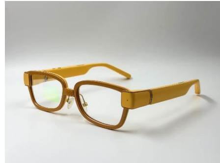
Figure 5. Picture of AR glasses made with 0.12" green micro-LED display. The resolution of the micro-LED display is 640 \times 480 .
