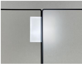
Figure 1. Comparison of AG in cover glass (Left: without AG, Right: with AG)
