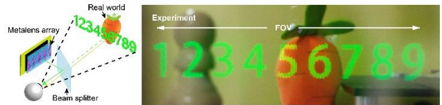
Fig. 5. Experimental result of FOV expansion: a 40-degree-FOV confirmed with a commercial camera
