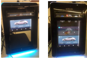
Figure 15. Panel image after environmental test such as rolling cycles of 200,000 at 25°C, 85°C/85% for 240 hours, and -40°C for 240 hours, respectively.
