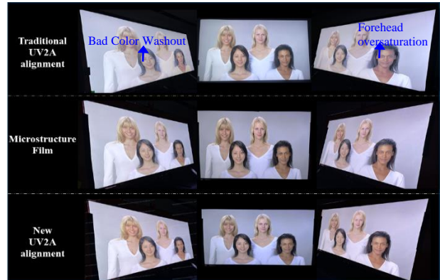
FIG. 10 The comparison results of the traditional UV2A alignment, the new UV2A alignment and the micro-prism structural film in the skin Color screen
