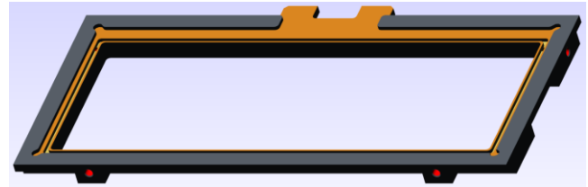
Figure 1. Frame for display fixation (extension for FPC shown on top side).
