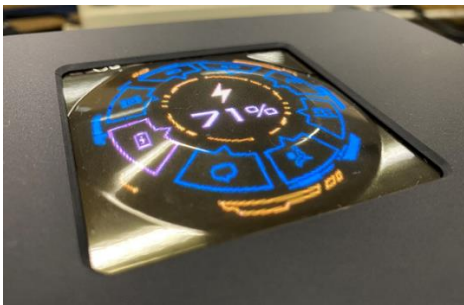
Figure 3. 3.5" stretchable MicroLED display with 141PPI
