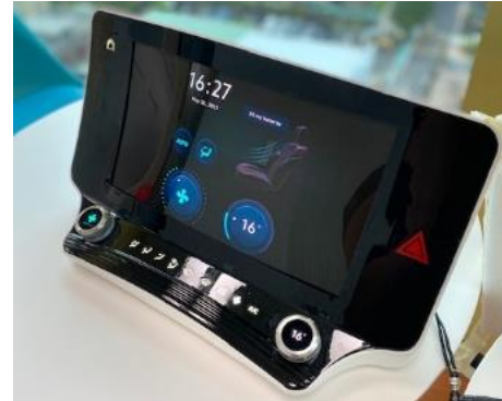
Figure 8. Photograph of a 13.8" stretchable MicroLED display.
