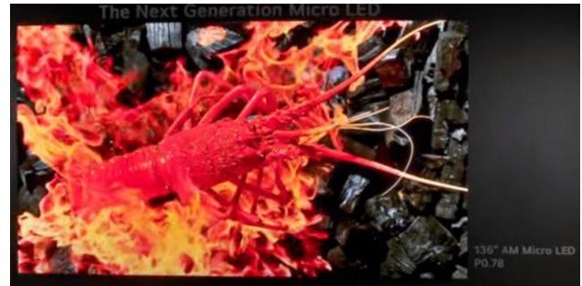
Figure 9. The image of 136" Seamless Tiling Micro-LED Displays with a resolution of UHD (3840x2160) and a pixel pitch of 0.78
