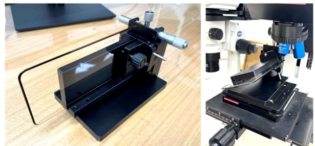
Figure 2. Micro-spectrophotometer of Olympus (USRM-RU-W) and a jig for tilting the sample at various angles to achieve perpendicular light incidence and reflection
