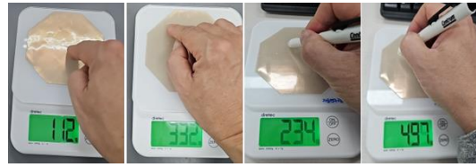
Figure 3. Evaluation of applied pressure on a stretchable panel to determine the reference load for scratch resistance testing.
