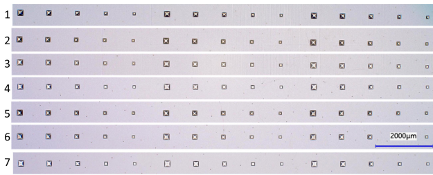
Figure 6. Seven designs of s/d with two types of well array arrangement and their respective five different scale sizes were capable of forming diaphragms.
