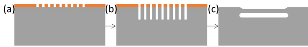
Figure 1. Schematic diagram of the process flow. (a) Lithography. (b) Dry etching. (c) Photoresist removal and annealing.
