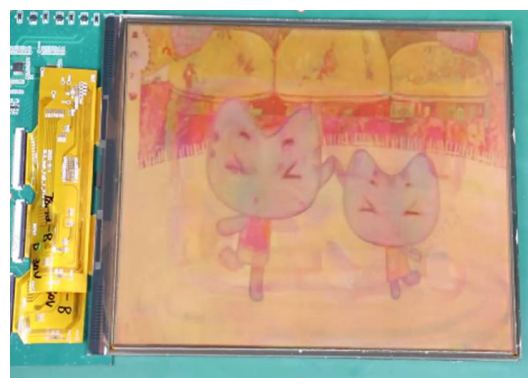
Figure 5. The electrowetting display EPD of 10.3 inch
