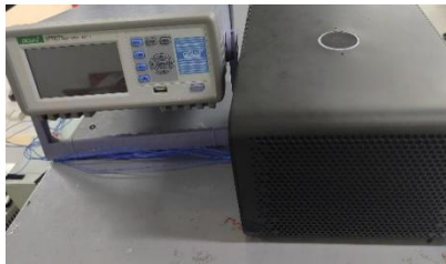
Figure10. Projection light machine temperature test platform.
