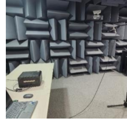
Figure11. Prototype noise test platform.
