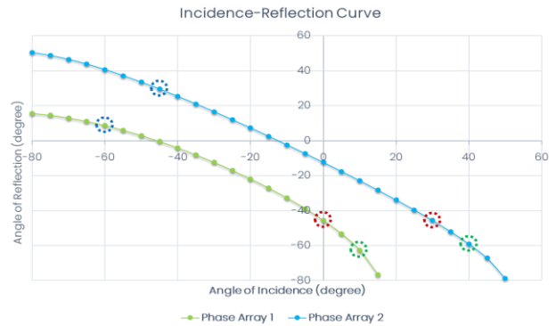
Figure 2. Incidence-Reflection relation of 2 phase arrays.
