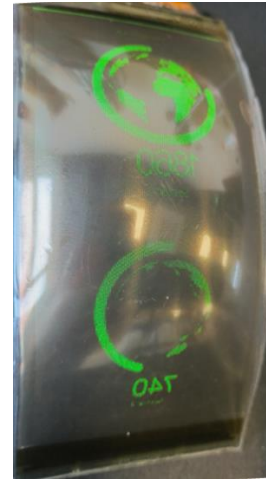
Figure 6. Photograph of 3D-stretched OLED display prototype.
