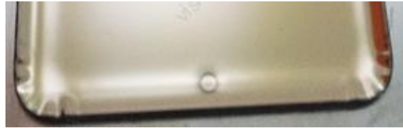
Figure 1. Wrinkles at the corners position on CG
