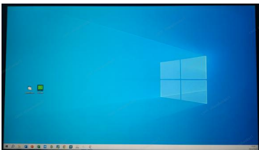
Figure 6. 14 inches notebook fabricated in G4.5 using polyimide B.
