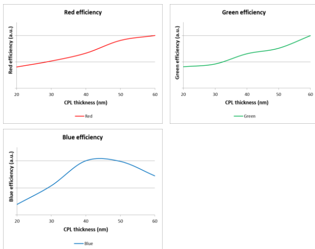
Fig. 9 Red, Green, Blue Subpixel Efficiency According to CPL Thickness
