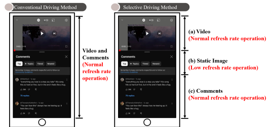
Fig 2. A schematic diagram of conventional driving and the proposed selective scan driving.
