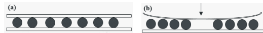
Figure 1. (a) Flexible Cell with BS (b) BS sliding or aggregation during high-pressure PVB lamination
