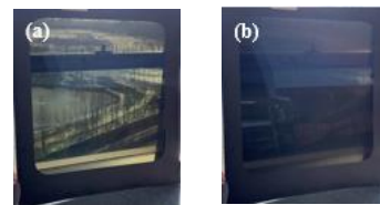
Figure 8. (a) Bright State at 27V (b) Dark State at 0V
