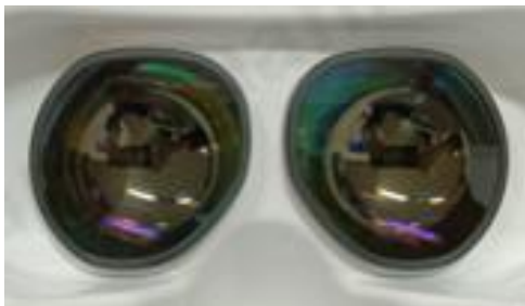
Figure 4 (b). The asymmetric prototype of VR lens
