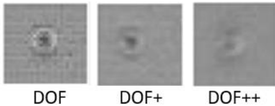
Figure 5. It is an actual product defect image according to the depth of field (DOF), and the blurring phenomenon increases toward the right.
