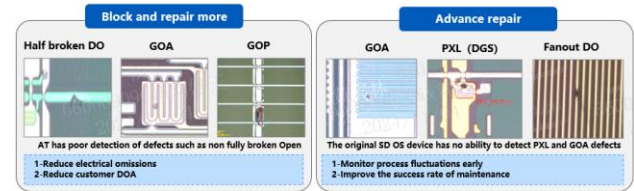
Figure 4. Multiple blockages, repairs and pre maintenance
