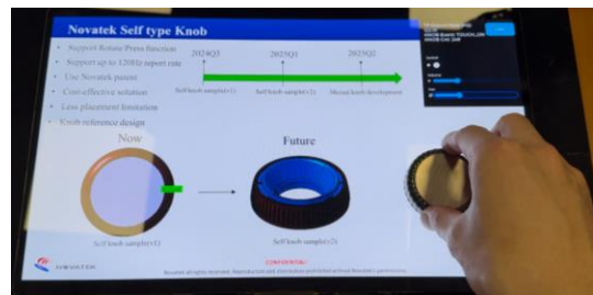
Figure 3. Knob manipulation demonstration on the in-cell touch LCD
