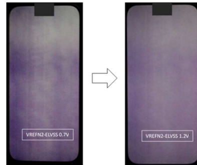
Figure 4. MURA compare between VREFN2-ELVSS 0.7V and VREFN2-ELVSS 1.2V
