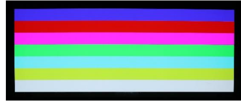
Figure 9. The image of the 16-inch LCD by using LTPS-TFTs with Al gate.
