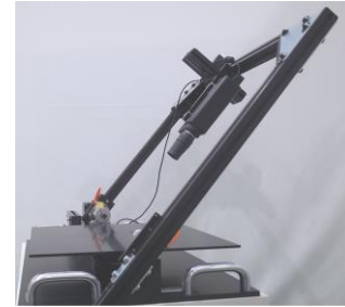
Figure 3. Colorimeter and rotation arm for color gamut measurement at various viewing angles.
