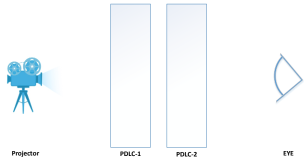
Fig. 1. System scheme of the multi-plane optical see-through volumetric 3D display system.
